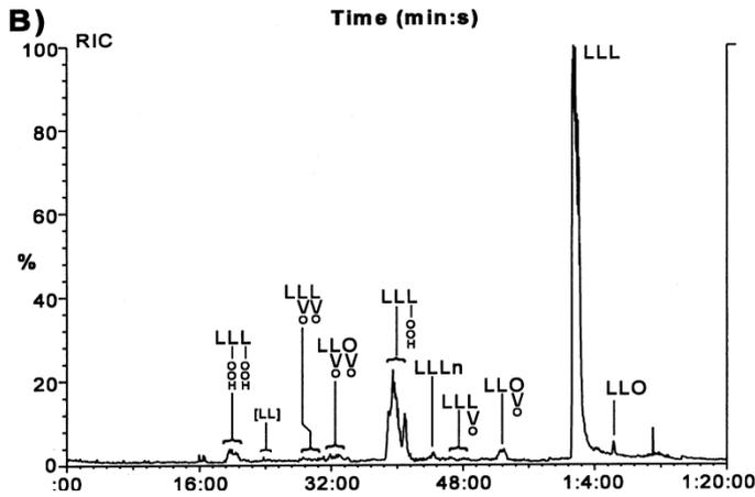
Fig. 4. HPLC chromatogram of autooxidized trilinolein and 1,2-dilinoleoyl-3-oleylglycerol.
